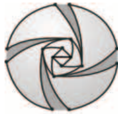
Fig. 5. A pointed rigidity circuit. The figure depicts one side of the sphere, the other side looks similarly.
