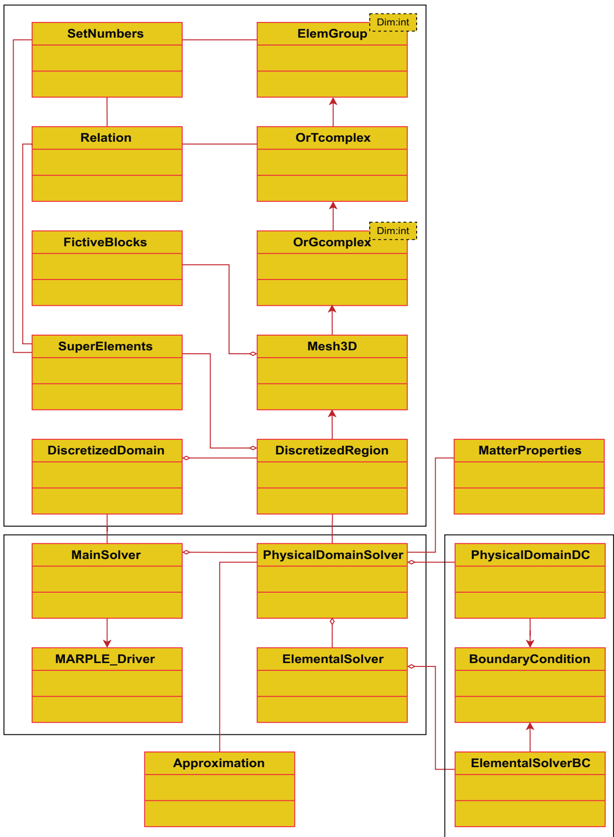
Figure 4. UML class diagram: architecture of MARPLE.
